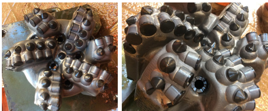
319m Drilled (32.7 hrs) Average ROP 9.76m/hr Dull 1-1-WT-A-X-I-NO-PP
