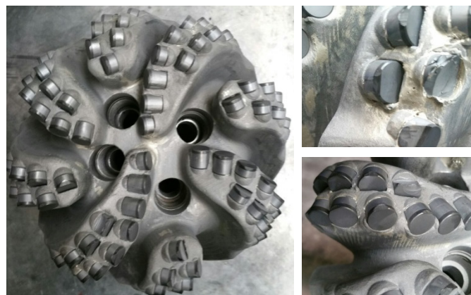
129m Drilled (35.00 hr) Average ROP 3.64 m/hr Dull 2-2-WT-A-X-I-CT-PR
